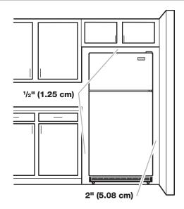
To ensure proper ventilation for your refrigerator, allow for a  $\frac{1}{2}$ " (1.25 cm) space on each side and at the top. Allow at least 1" (2.54 cm) between back of cabinet and the wall. If your refrigerator has an ice maker, make sure you leave some extra space at the back for the water line connections.
