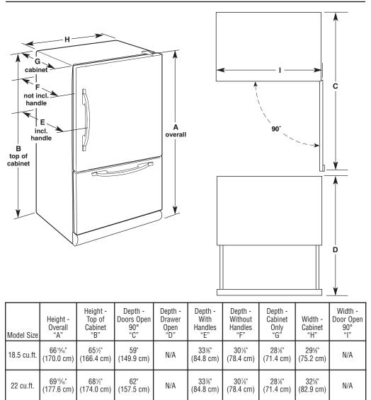
To ensure proper ventilation for your refrigerator, allow for a  $\frac{1}{2}$ " (1.25 cm) space on each side and at the top. Allow at least 1" (2.54 cm) between back of cabinet and the wall. If your refrigerator has an ice maker, make sure you leave some extra space at the back for the water line connections.
