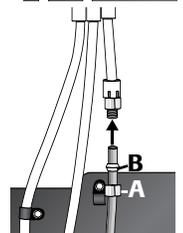
4. Place end of copper tubing into water valve inlet port. Shape tubing slightly. **Do not** kink – so that tubing feeds straight into inlet port.
