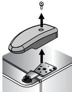
4. Unscrew  $\frac{5}{16}$ " hex head screws from top hinge to remove hinge and retain all screws for later use.
