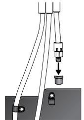
3. Place brass nut (A) and sleeve (B) on copper tube end as illustrated.
