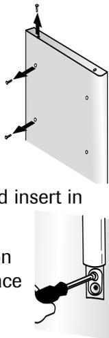
3. Locate handle trim in literature pack and install over top and bottom of handle, as illustrated.
