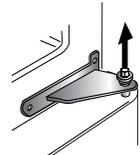
8. Remove bottom hinge or stabilizing bracket with  $\frac{3}{8}$ " hex head driver and retain screws for later use. Lift out bottom hinge pin (on freezer door models).
