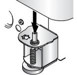
3. **Freezer door models:** Place hinge side of freezer door on bottom hinge pin and hold freezer door upright while installing center hinge pin with  $\frac{5}{16}$ " hex head driver.
