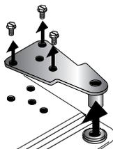
7. Remove Phillips screws to remove center hinge and retain all screws for later use.
