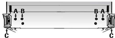
3. Using the hex head driver, turn each of these adjustment screws **(B)** to raise or lower the rear of the refrigerator.
