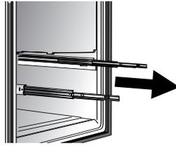
2. While supporting door front, hook supports into tabs located on inside of rail.
