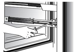
6. Lift top of drawer front to unhook supports from rail system. Lift door front out to remove.
