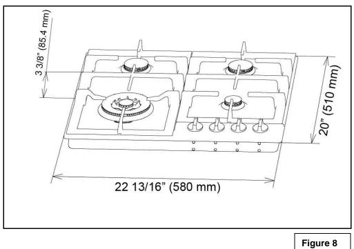
Cut the opening in the countertop. To ensure accuracy it is best to make a template (see Figure 9) for the opening. Make sure the sides are parallel also rear and front cuts are exactly perpendicular to the sides. Observe all minimum clearances.
