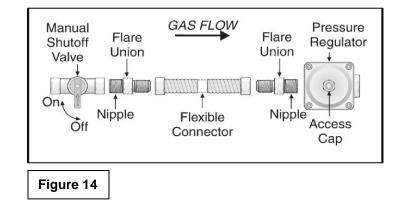
tightening may crack the regulator resulting in a gas leak and possible fire or explosion (see Figure 14).
