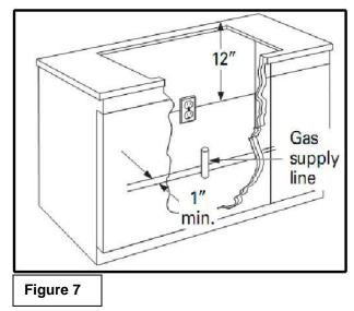
• The electric spark ignition feature for this model requires a 120V electrical power supply and should be located 12" below the countertop and within reach of the cooktop's four-foot power cord.
