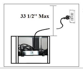
Place the outlet at a maximum distance of 33 1/2" from where the cord exits on the hood
