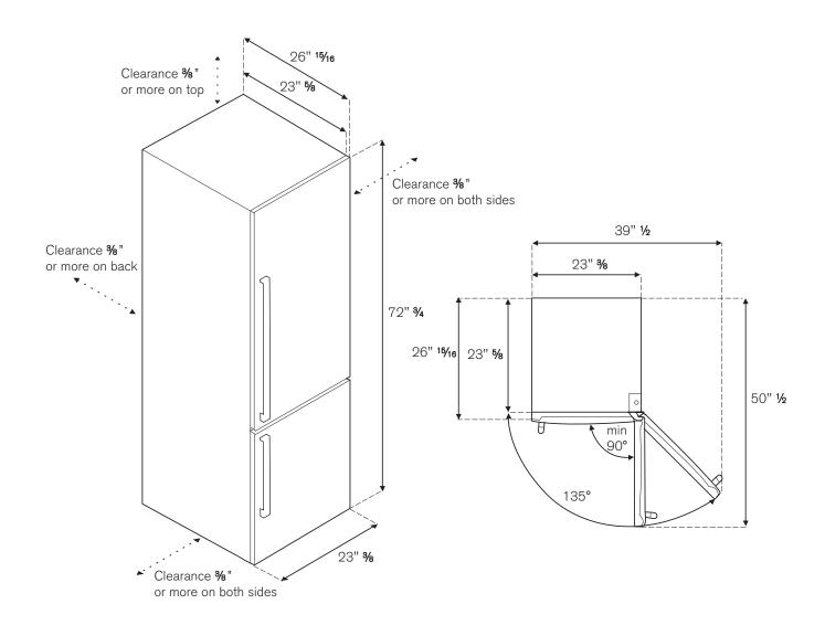
INSTALLATION: There shall be a space not less than 3/8 inch from the top of your refrigerator, not less than 3/8 inch from both sides and 3/8 inch or more from the back of the refrigerartor to the adjacent walls respectively. This requirement is necessary to create clearance in order to open and close the door as well as to avoid the spacing for adequate ventilation around the refrigerator.
