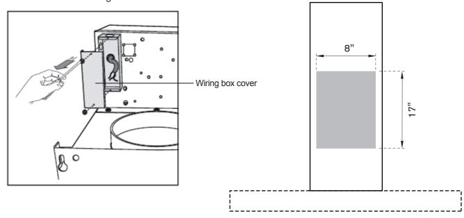
If the power cord to connect the hood to the main power comes from the wall in the grey area (8"x17"), it must have a minimum length of 20" to be connected to the Junction Box.
