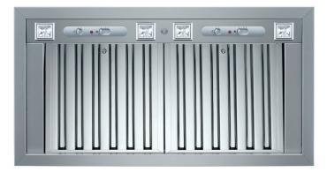
For use with custom canopies, this high-performance insert hood with baffle filters has two motors controlled by three settings for different extraction levels. Four halogen lights give exceptionally bright worktop illumination. The removable filter elements are dishwasher safe.
