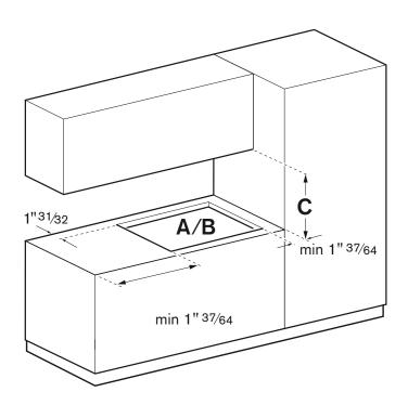
C = 30" (76.2 cm) minimum clearance between top of cooktop platform and bottom of uncovered wood or metal cabinet (24" [61 cm] minimum clearance if bottom of wood or metal cabinet is covered by not less than 1/4" [0.6 cm] flame retardant millboard covered with not less than 1/4" [0,6 cm] flame retardant millboard covered with not less than No. 28 MSG sheet steel, 0.015" [0,04 cm] stainless steel, or 0.024" [0.06 cm] aluminum or 0.020" [0.05 cm] copper).
