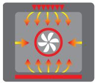
The European convection system and 4 usable shelf positions ensure even heat roasting and baking on multiple levels with no flavor crossover.
