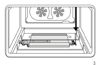
Unscrew the nozzle located inside the gas fitting using a 7 mm [socket wrench].
