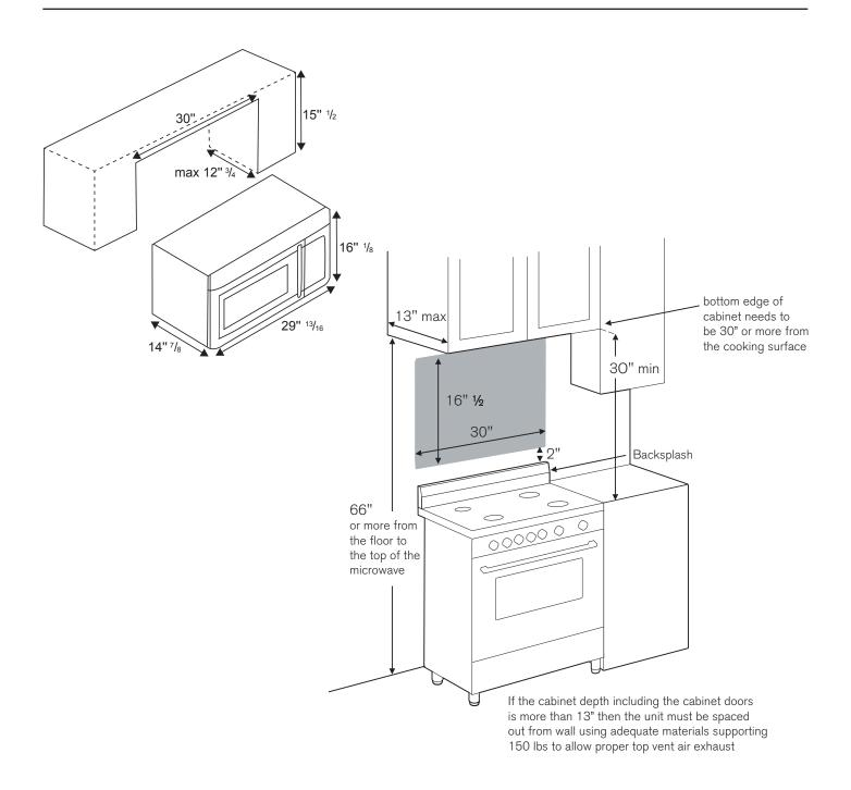
Bertazzoni recommends to operate the appliance after it has been installed in a cabinet. The kitchen cabinets shall be made of materials capable of withstanding temperatures at least 117°F (65°C) above room temperature in order to avoid possible damage to the cabinets during oven usage. For further installation instructions refer to the installation manual.
