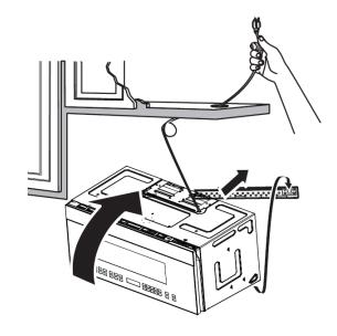
Bertazzoni recommends to operate the appliance after it has been installedin a cabinet. The kitchen cabinets shall be made of materials capable of withstanding temperatures at least 117°F (65°C) above room temperaturein order to avoid possible damage to the cabinets during oven usage.
