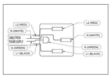
Fig. 7 FOUR-WIRE CONN.RECEPTACLE NEMA 14-50R
