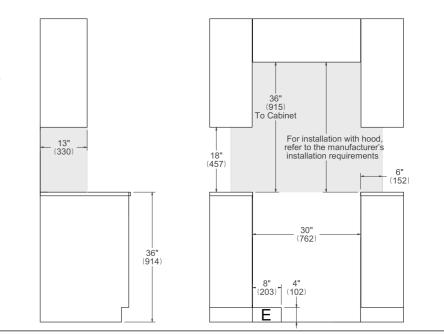
NOTE a. Electrical Connection b. Gas Connection
