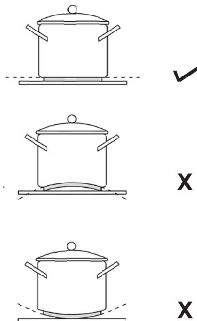
Pans that are not completely flat and have a recessed bottom leave an air gap between pot and cooktop, which during operation can reach very high temperatures that can damage the glass top and the inductors below the glass.
