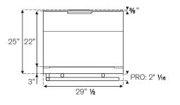
INSTALLATION: There shall be a space not less than 1 inch from the top of your refrigerator, not less than 1/4 inch from both sides and 1 inch or more from the back of the refrigerartor to the adjacent walls respectively. This requirements is good for open and close of the door and also for heat emission.
