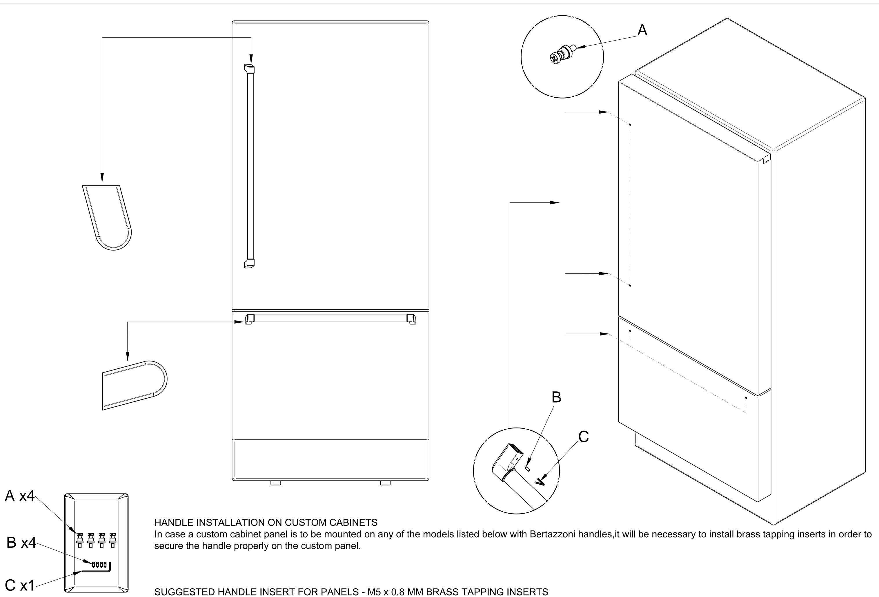
Recommended drill bit size to drill the pilot hole is 3/8" Suitable inserts can be ordered at www.encompassparts.com Part Number: 95631A100, contains n°4 M5 brass hardwood inserts and 1 M5 installation bit Do not use a power tool to mount the inserts. Installation of the inserts with improperly calibrated power tools risk damaging the panels.
