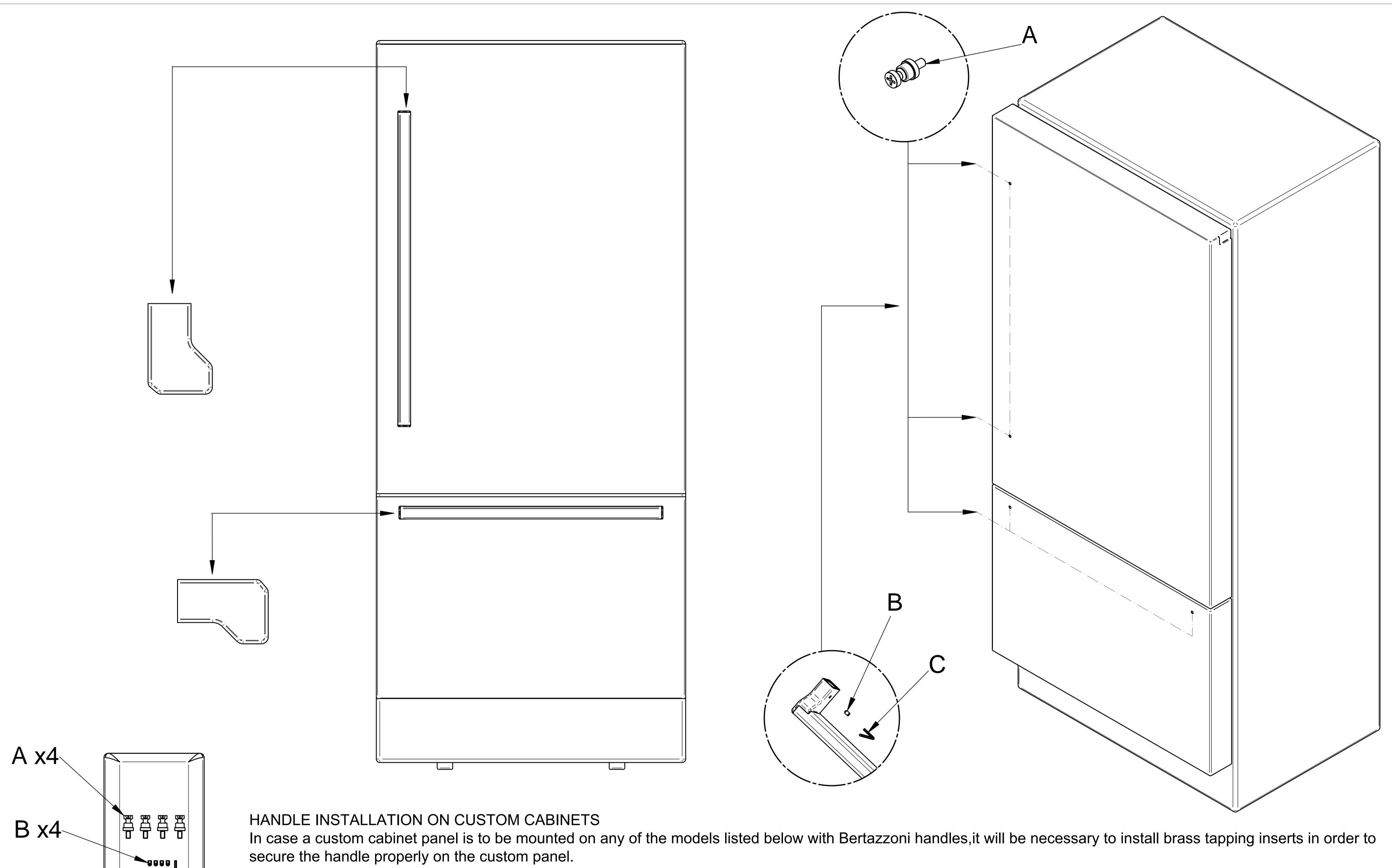
SUGGESTED HANDLE INSERT FOR PANELS - M5 x 0.8 MM BRASS TAPPING INSERTS Recommended drill bit size to drill the pilot hole is 3/8" Suitable inserts can be ordered at www.encompassparts.com Part Number: 95631A100, contains n°4 M5 brass hardwood inserts and 1 M5 installation bit Do not use a power tool to mount the inserts. Installation of the inserts with improperly calibrated power tools risk damaging the panels.
