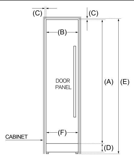
NOTE: The freezer comes with a 4" (100 mm) stainless steel toe kick installed to fit a standard 84" (2134 mm) tall cabinet niche. For flush installation in a standard 25" (635 mm) deep cabinet niche, maximum door panel thickness is 15/16" (24 mm).
