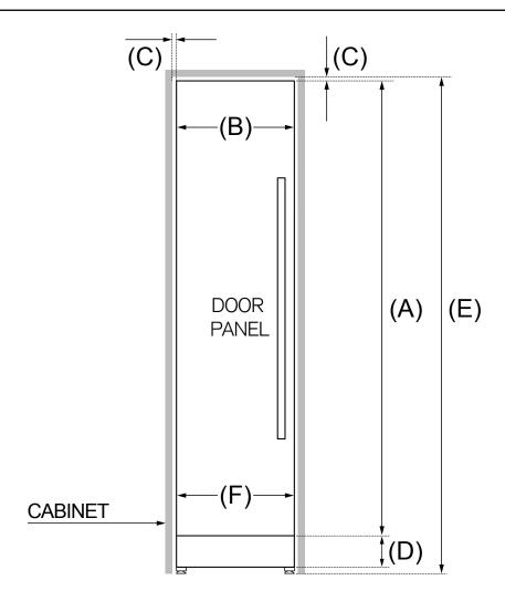
NOTE: The refrigerator comes with a 4" (100 mm) stainless steel toe kick installed to fit a standard 84" (2134 mm) tall cabinet niche.
