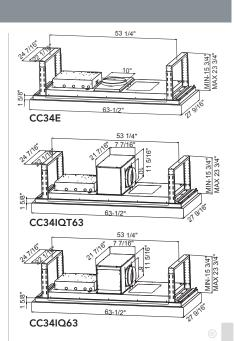
Installation height above the cooking surface 48" minimum, 72" maximum recommended.
