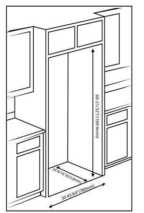
Required Minimum Clearances: Top: 2" Sides: 1 <sup>37</sup>/<sub>64</sub>" on each side Back: 2"
