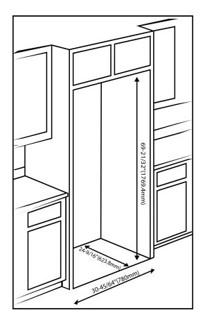
Required Minimum Clearances: Top: 2" Sides: 1 <sup>37</sup>/<sub>64</sub>" on each side Back: 2"
