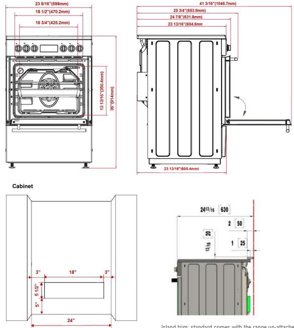
**Required minimum air gap clearances:** <sup>1</sup>/<sub>4</sub>" sides
