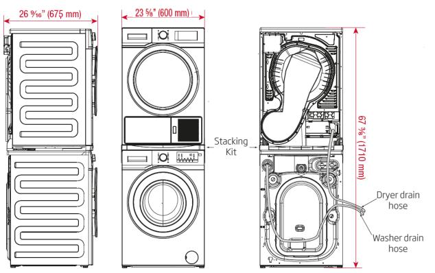
Stacked installation minimum air gap clearances: 6 ¼" top, ½" sides, ½" back, front ½"
