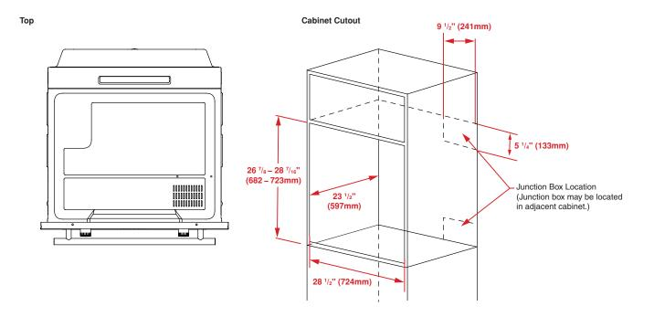
If installing in lower cabinet, leave 4" (102mm) min clearance below.
