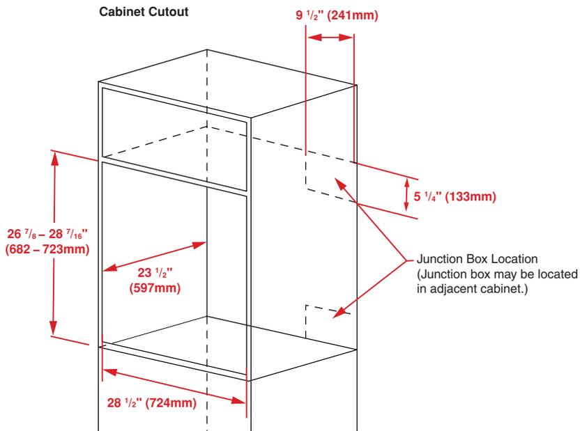
If installing in lower cabinet, leave 4" (102mm) min clearance below.
