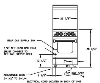
LOCATION OF ELECTRICAL OUTLET MUST NOT BE HIGHER THAN 3" FROM FLOOR IF LOCATED BEHIND THE UNIT OR CAN BE LOCATED IN AN ADJOINING CABINET.
