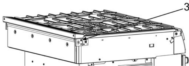
Figure 7 : Garniture d'îlot installée
