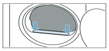
Separate the two-part lint filter and open both parts as shown.
