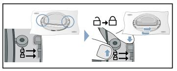
**9.** Place the hook insert in position adjacent to the handle slots/openings and the hinge insert in the opposite position as shown. Reinstall the original screws.
