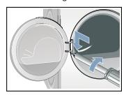
**14.**Confirm the door closes and latches in place. Plug in the dryer to operate it.
