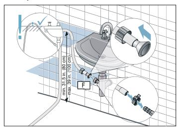
Minimum height of drain for installation shown above is 31.5 in. (80 cm). Maximum height of drain is 39 in. (100 cm).
