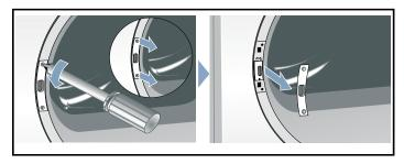
**11.**Remove the door latch from the dryer housing.
