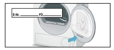
The **E-Nr.** (model number) and the **FD** (serial) number can be found on the rating plate label (shown above) or in the Home Connect application under Appliance Information.
