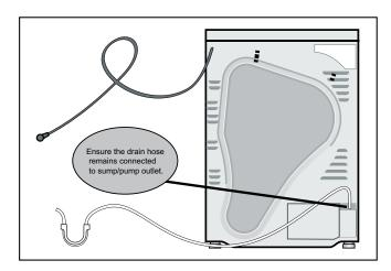
**NOTICE:** Do not reuse an old or different drain hose. Only use the drain hose included with the dryer.
