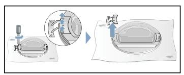
**5.** Remove screws from the hook insert and then remove it from the door.
