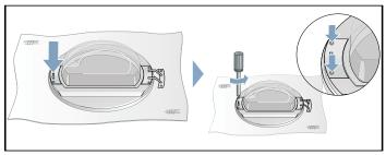
**10.**Remove screws from the door latch cover and then remove it from the dryer housing.
