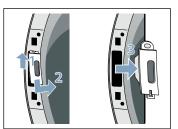
**12.**Install the door latch (1) and then door latch cover (2) on the opposite side of the door opening.
