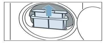
The filters should be cleaned after or before every drying process. Cleaning the filters reduces the drying time and saves energy.
