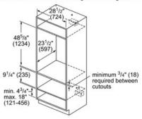
\* Wall oven junction box may be located above or right or left of the unit within reach of the power conduit.
