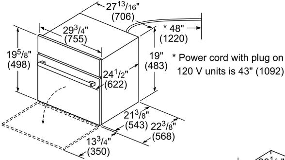
**IMPORTANT: Bosch Speed Oven is not approved to be installed under a cooktop.**
