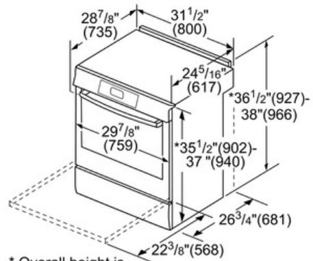
\* Overall height is adjustable via leveling legs.
