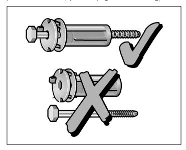
☐ Store the transport bolts with the washer and bush attached.
