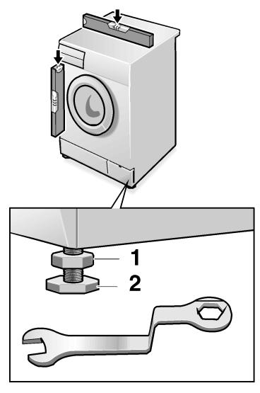
Level the washing machine with the assistance of the four adjustable feet and a spirit level:
