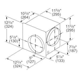
measurements in inches and (mm)
