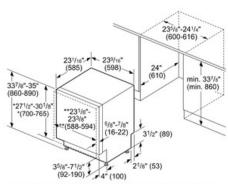
measured from the bottom edge of the countertop panel thickness recommended 3/4\* (20 mm), panel weight 7-22 lbs (3-10 kg)
