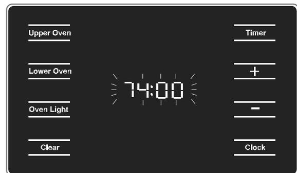
5. Press **+** or **-** to edit Sabbath cook time by 30 minute increments. Holding the button more than 1 seconds causes the displayed value to change 30 minutes each 1/2 second until the button is released. The maximum time allowed to be set is 74 hours.
