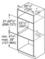
\* For single ovens installed into a wall cabinet, the junction box may be located above or beneath the unit within reach of the power conduit.
