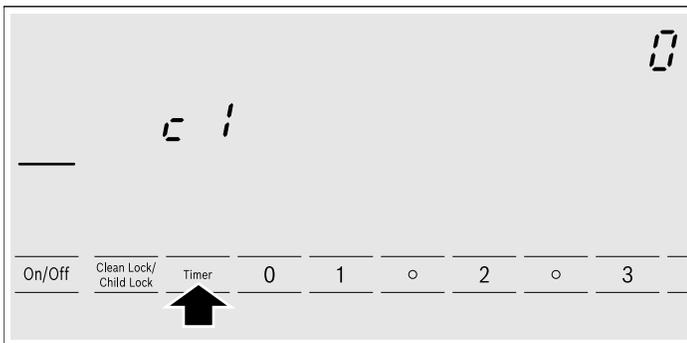
3. Touch the **Timer** key until the indicator for the required function is displayed.
