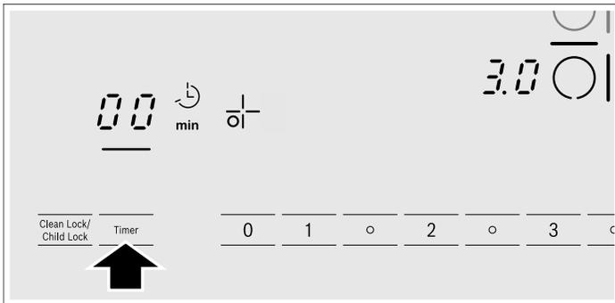
3. Within the next 10 seconds, set the required time using the number keys **1** to **9**.
