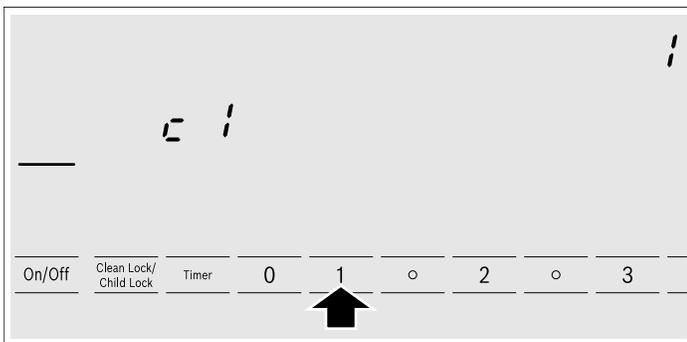
5. Touch the **Timer** key again for 4 seconds, until you hear a sound signal. The settings have been correctly stored.
