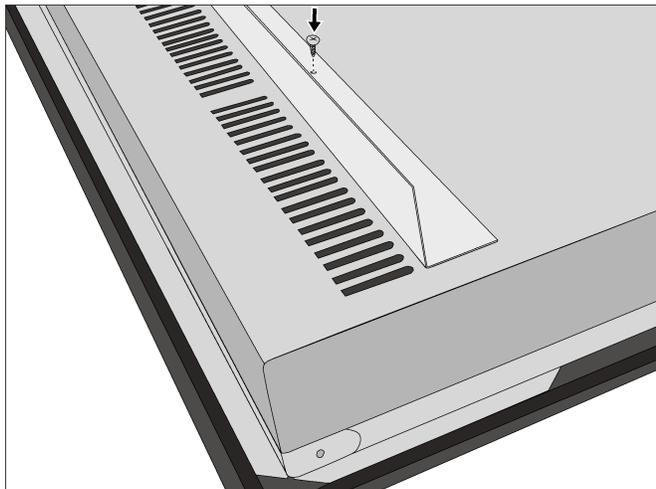
Screw the heat shield to the base of the burner box using the pre-drilled holes, as shown in the illustration.
