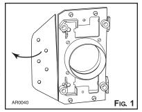
pieces as you join them to spread the cement, and align the mounting plate in a vertical position.
