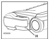
and turn it over to see if there is an obstruction. When brush roll jam has been cleared, press the reset button (**H**) and connect the power brush back to the wand. Finally, turn the power unit/power brush back on. If it fails to restart or continues to trip without any apparent reason, the power brush must be serviced by an authorized service center.
