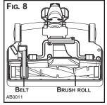
To free brush roll from base, start by sliding the belt side end and pull brush roll sideways (1). Once disengaged from housing, lift brush roll (2) out of its compartment (Fig. 9).
