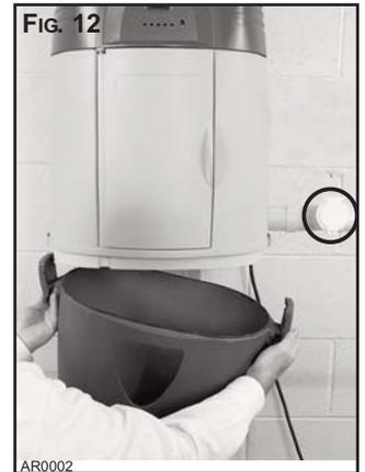
Utility valve (circled in Fig. 12), next to power unit, can be used to service area around where power unit is installed.
