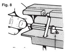
Reinstall pedal by matching it up and sliding hinge pin through one hinge bracket. (Fig. 8)
