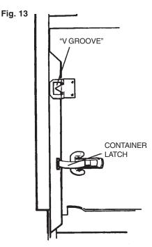
Bag is locked between door flange and drawer. When door is closed and latched properly, door guide "V" will be snug in "V" groove in drawer flange. (Fig. 13)
