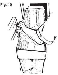
With the drawer extended to the second stop, release the container latch and swing open door. Then slide bag into drawer from front to back. Starting at the back of the drawer, fold bag over top rim of drawer on all sides. (Fig. 10)
