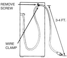
For free-standing unit, remove wire clamp to obtain additional cord length if necessary. (Fig. 3)
