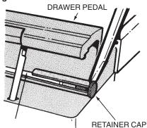
2. With a commonhead screwdriver pry off the retainer cap on each end of the drawer pedal. (Fig. 4)
