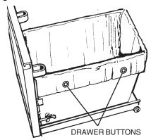
Smooth and shape the bag carefully this will prevent the bag from being torn by the ram during compaction. Using buttons on side of drawer, button your bag in place by using the prepunched holes in the side of the bag. Figure 12 shows the bag installed.
