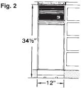
Your compactor has been designed to require a minimum of space whether free-standing or built-in. Only 12" wide x 20" deep, your compactor is smaller than most on the market. (Fig. 2)
