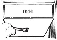
Remove bolt in center of ram with 1/2" wrench. (Fig. 15)
