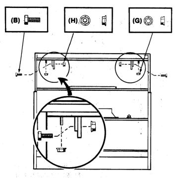
3. Attach hood to rough-in plate with two screws and nuts. Install one lock nut on each vertical adjustment stud at top of hood.
