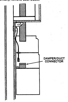
Place hood in position and drop power cord through opening in back of hood. If ducting vertically, slide duct over damper/duct connector.
