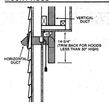
1. Check duct length. Duct should end 14-3/4" below top of rough-in plate for 30" high hood. If ducting horizontally, remove duct elbow.
