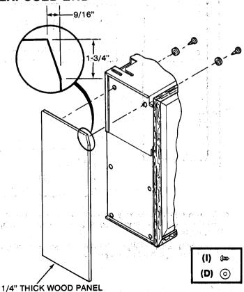
1. Attach a 1/4" thick end panel with six screws and washers and notch for frame clearance, as shown.
