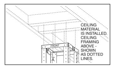
After ceiling surface is finished, align frame assembly to ceiling framing, and attach to ceiling framing with (6) 4mm x 38mm screws. Tighten securely, making sure that the upper frame bracket is tight against the ceiling.
