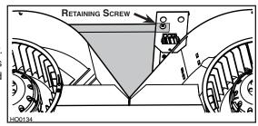
Single Blower Unit: Position the power pack below the installed custom hood. Insert the house wiring cable through the wire clamp previously installed in step 10. Tighten the wire clamp to secure the cable.
