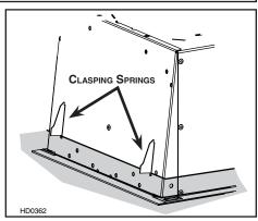
From inside the power pack, using provided no.  $8-10 \times 1/2$ " screws, mount the power pack to the custom hood base. To do so, lift one side until its flange rests on the outer side of the custom hood base and use 2 screws to secure in place.
