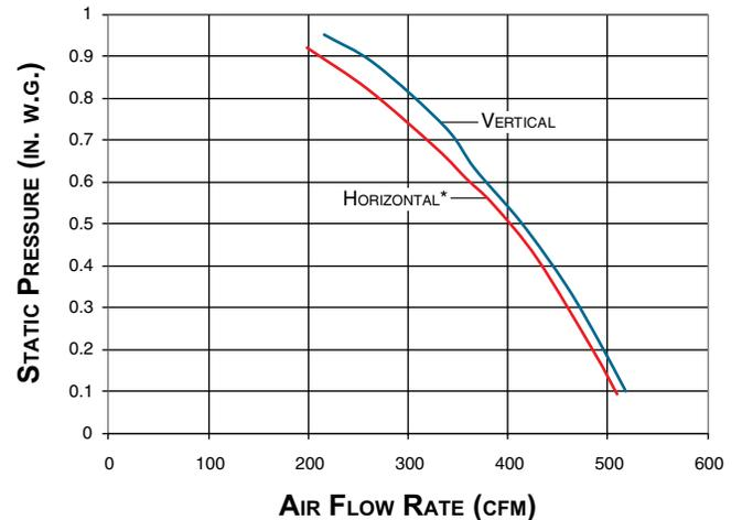
\* ALTHOUGH THE HORIZONTAL DISCHARGE INSTALLATION IS FEASIBLE, THIS INSTALLATION TYPE SHOULD BE ONLY PERFORMED IN SPECIFIC SITUATIONS SINCE IT REQUIRES PARTICULAR KNOWLEDGE AND TECHNICAL SKILLS FROM THE INSTALLERS.
