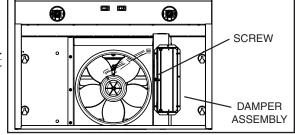
Remove the wiring cover (shaded part in illustration at right) retaining screw. Set aside the <u>Wiring Cover</u> and its screw.
