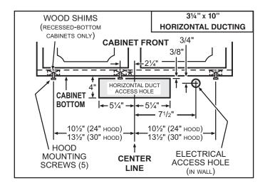
\* Note the extra wood shim and mounting screw near the cabinet front.
