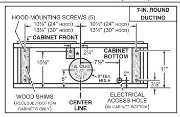
\* Note the extra wood shim and mounting screw near the cabinet front.
