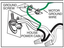
Reinstall wiring cover and attach it to the hood using its retaining screw.
