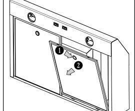
Using the finger cup, remove the <u>Grease Filters</u> from the hood by pushing down **1** and tilting filters out **2**.
