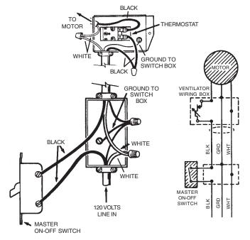
For standard installation, connect the two leads in the thermostat wiring box to the two power leads. Attach ground wire from the power cable to the green screw in the box.
