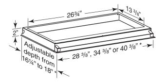
\* Exterior depth and width dimensions do no include 3/8" wide flanges.
